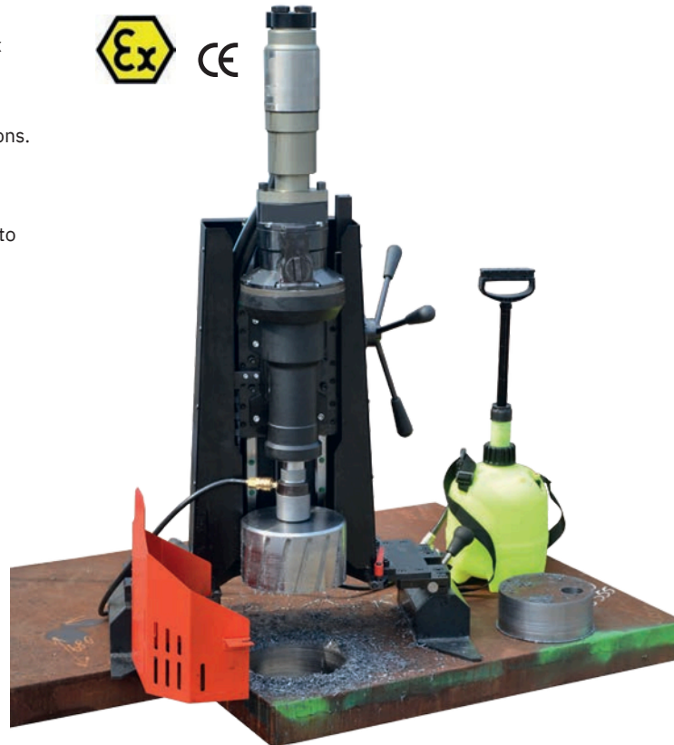
200 mm Ø cutter capacity
