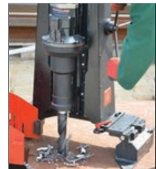
45 mm Ø solid drill capacity
