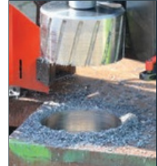
200 mm Ø cutter capacity
